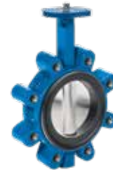
Series 820/10 Butterfly valve Centric with loose liner Lug type DN25-600 PN10/16 Ductile iron
