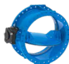
Series 756/106 Butterfly valve Double eccentric Welded stainless steel seat IP 68 gearbox DN150-1400 PN10/16 Ductile iron
