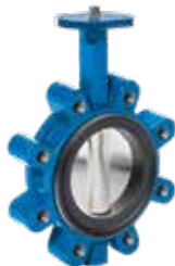
Series 820/10 Butterfly valve Centric with loose liner Lug type DN25-600 PN10/16 Ductile iron Options: • for frequent operation • U-section type • various actuators
