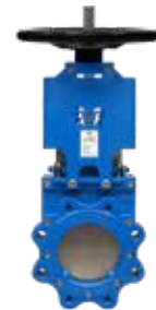
Series 702/20 Knife gate valve with handwheel and rising stem DN50-1200 PN10 Ductile iron Options: • handwheel and non-rising stem • chainwheel • electric or pneumatic actuator • lever
