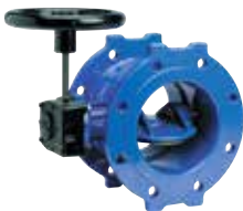
Series 756/100 Butterfly valve Double eccentric Double flanged Integral seat IP 67 gearbox DN150-2800 PN10/16 Ductile iron
