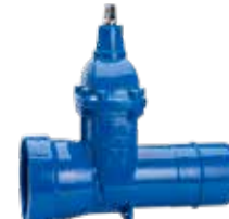
Series 33/50 Gate valve with BLS® socket end/ BLS® spigot end for cast iron pipes DN80-300 PN16 Ductile iron
