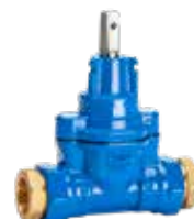
Series 03/30 Service connection valve with tensile socket ends for PE pipes DN20-50 PN16 Ductile iron
