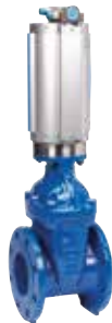
Series 715 Flanged gate valve with hydraulic actuator Face-to-face DIN F4 DN65-300 PN10/16 NBR wedge Ductile iron Options: • solenoid valve kit and proximity switches
