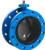
Series 75 Butterfly valve Centric with fixed liner Double flanged short DN50-2000 PN10/16 Ductile iron Options: • double flanged long • various actuators
