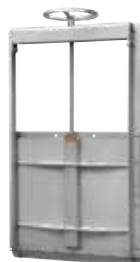
Series 772/61 Wall penstock Bi-directional up to and incl. 1200 x 1200 mm, in larger sizes bi- or uni- directional With non-rising stem Stainless steel AISI 304 200 x 200 mm - 2000 x 2000 mm Options: • rising stem • AISI 316
